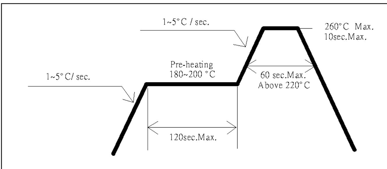
\*Recommended soldering conditions vary according to the type of LED
