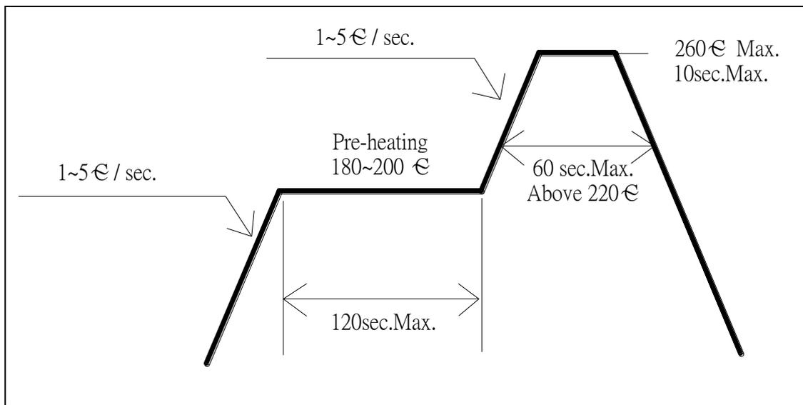
\*Recommended soldering conditions vary according to the type of LED
