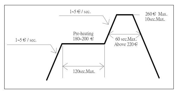
\*Recommended soldering conditions vary according to the type of LED
